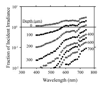
Fig. 2 Spectral attenuation: each spectrum shows the fraction of incident radiation in the soil at various depths (given in  $\mu$ m). *Filled and empty circles* are alternated to aid in reading the figure (adapted from Garcia-Pichel and Belnap 1996)
